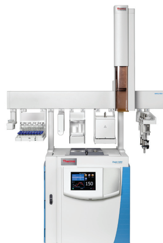
Figure 8. Greenhouse gas analyser with Head Space sampler for water, soil or organic material samples. Sample trays for up to 1 liter vials are optional available.
